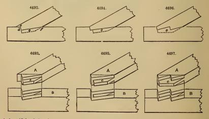
the whole width of the cheeks, in addition to that of the tenon ; and the notch so formed is called a joggle. Fig. 4693 shows the parts detached and in perspective. It will be seen that a much larger bearing surface is thus obtained.
